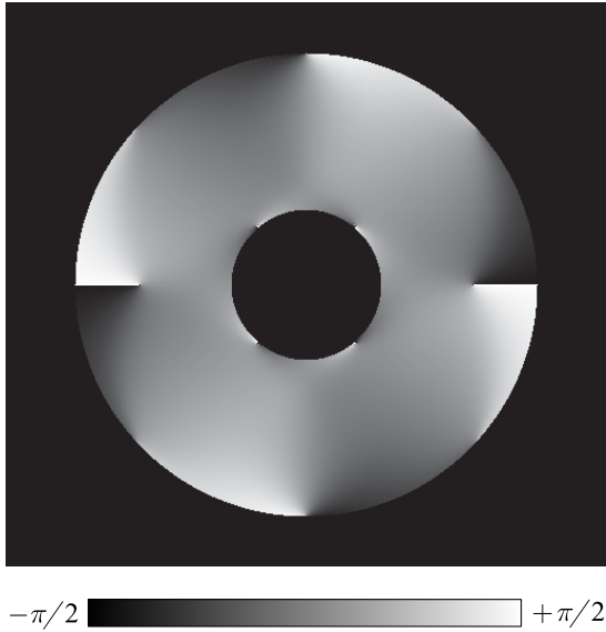
Fig. 5. Numerical map of unwrapped isoclinics in the range (-\pi/2, +\pi/2] computationally obtained from the phase unwrapping technique [3].
