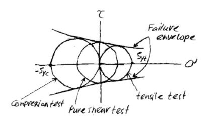
• <u>Coulomb-Mohr theory</u>: it assumes the failure envelope to be a <u>straight line</u>, thus shear test is not needed (*only tension and compression tests*).
