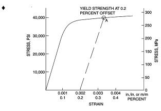
The slope of the linear portion of the curve equals the modulus of elasticity.
