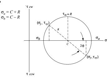
The maximum *inplane* shear stress is  $\tau_{in} = R$ . However, the maximum shear stress considering three dimensions is always
